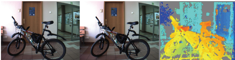
Fig. 3. Stereovision scene reconstruction - the left and right images and the result of the reconstruction; Grey areas represent pixel groups for which proper depth estimation was not possible
